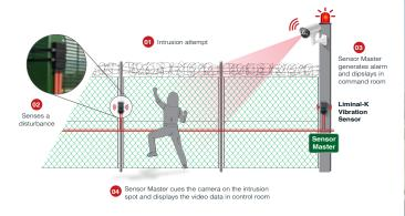
> Software: A-1 VIGIL can be integrated with industry leading surveillance monitoring softwares which helps in converting the sensor data into useful video output.
